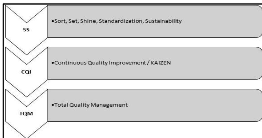
Figure 3: 5S-CQI-TQM approach to quality improvement
